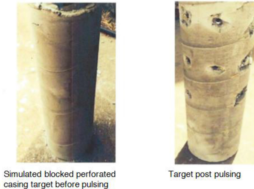
Fig. 4. Effect of PPT on the cement integrity after and before its application. 1
